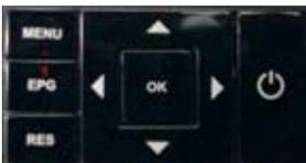
You can also use the front panel buttons of the ADB 5810 set top box to replace the basic remote control functions. Use **MENU** to display the Main Menu, **EPG** to display Guide, **RES** to change screen resolutions, and the **arrow** and **OK** buttons as you would those on the remote control.
