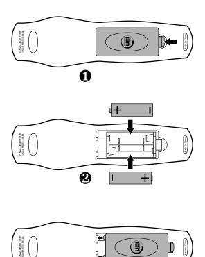
1. On the back of the remote control, push the tab and lift off the battery cover.
