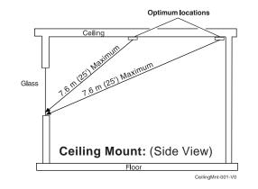
NOTE: If the device is ceiling mounted, the end with the hole (Microphone end) should face the protected glass.
